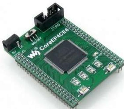
Fig.2 The FPGA core board.
